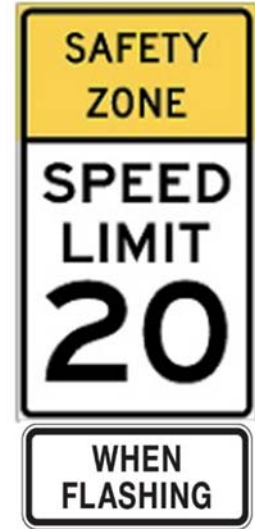
Figure 4: Safety Zone Speed Sign
