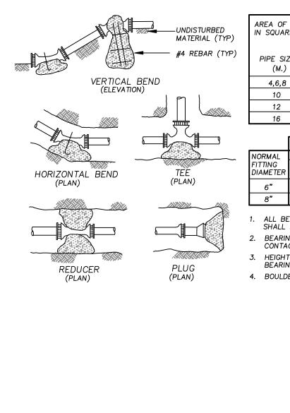
AREA OF BEARING FACE OF CONCRETE THRUST BLOCKS IN SQUARE FEET BASED ON 250 P.S.I. & 1.5 TONS/S.F. ALLOWABLE SOIL BEARING CAPACITY
