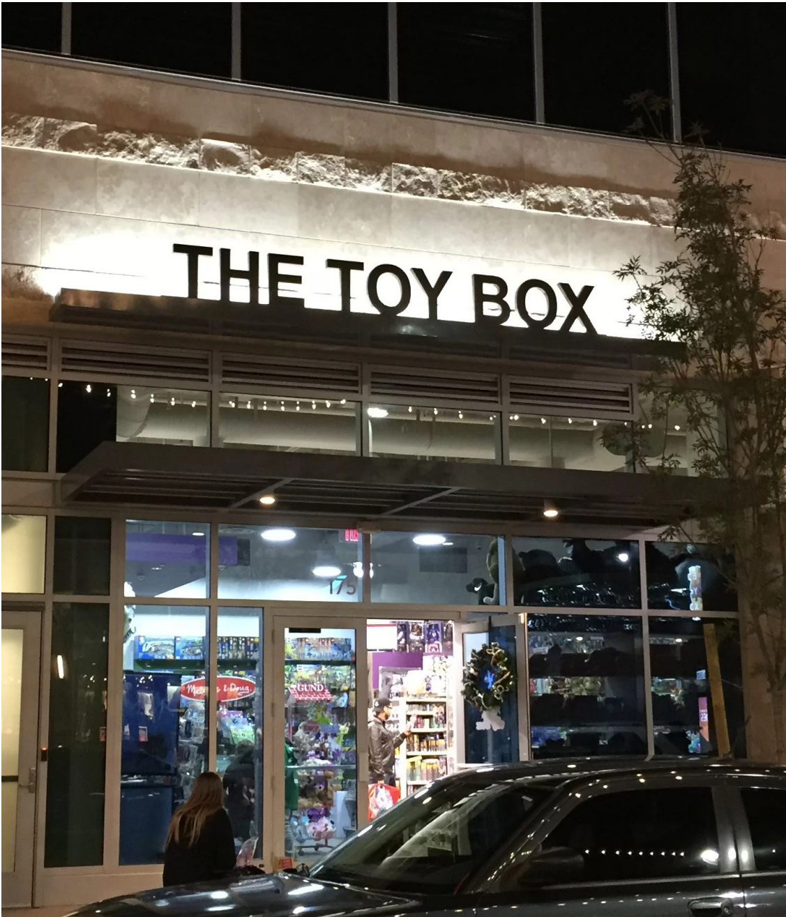
Storefront Sign Lighting Highlight store signage at night. Direct lighting only on sign and not adjacent sidewalk
