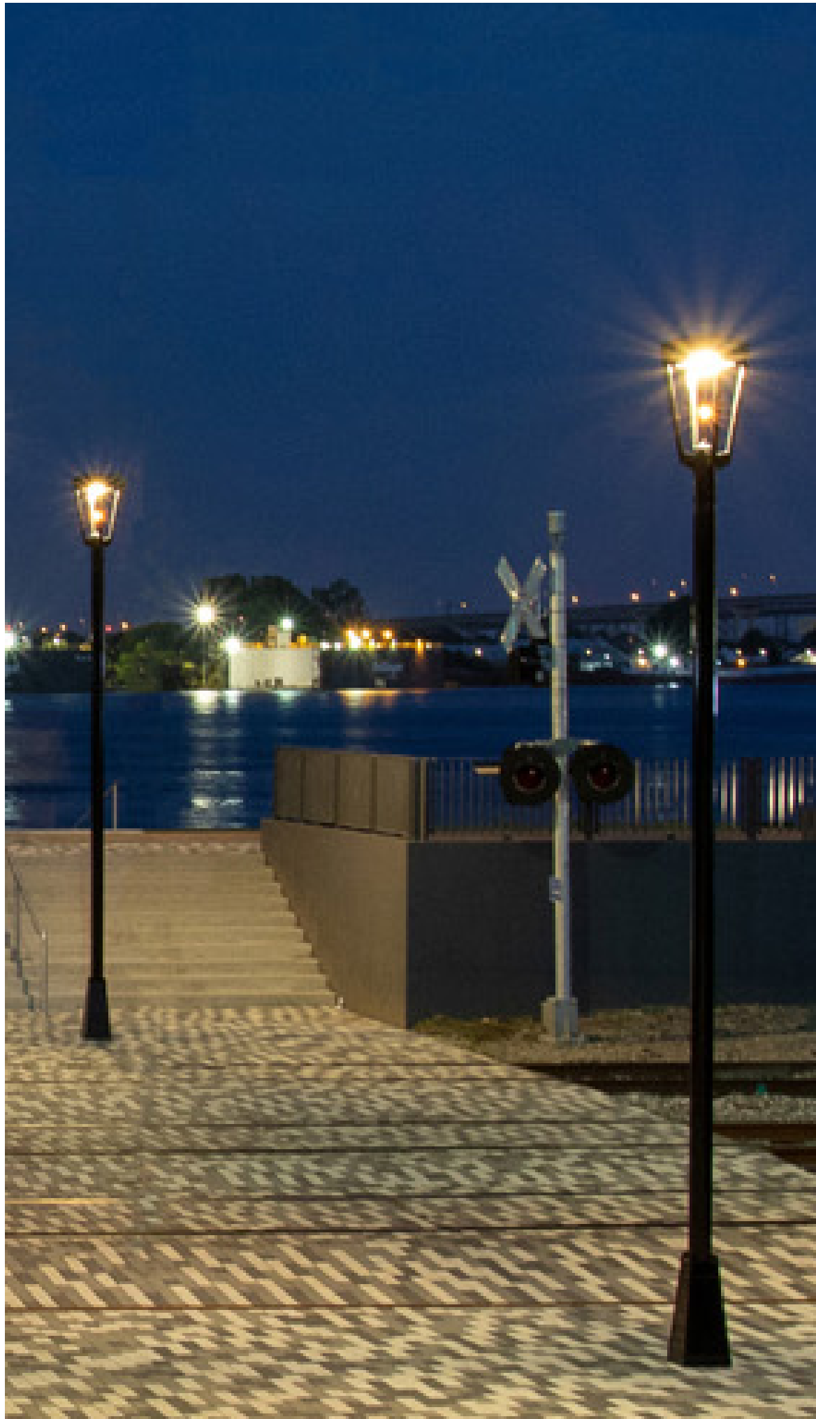
Pedestrian Scale Lighting Pedestrian scale lighting consists of light poles that are shorter than roadway light poles. Typically, they are less than 18’ tall. Pedestrian light poles are located within the right-of-way and are used to illuminate primarily pedestrian areas like sidewalks. Pedestrian light poles can be separate from roadway light poles or combined on the same structure.
