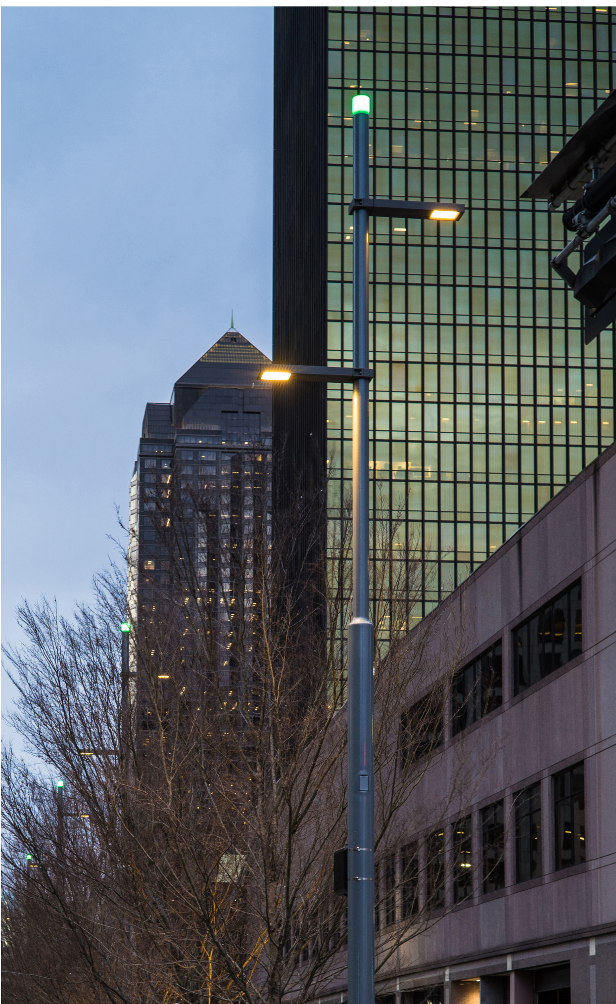
Combined Pedestrian and Roadway Lighting Combine pedestrian and roadway lighting on single utility pole. Route 20 roadway lighting must follow the standards set by the state.
